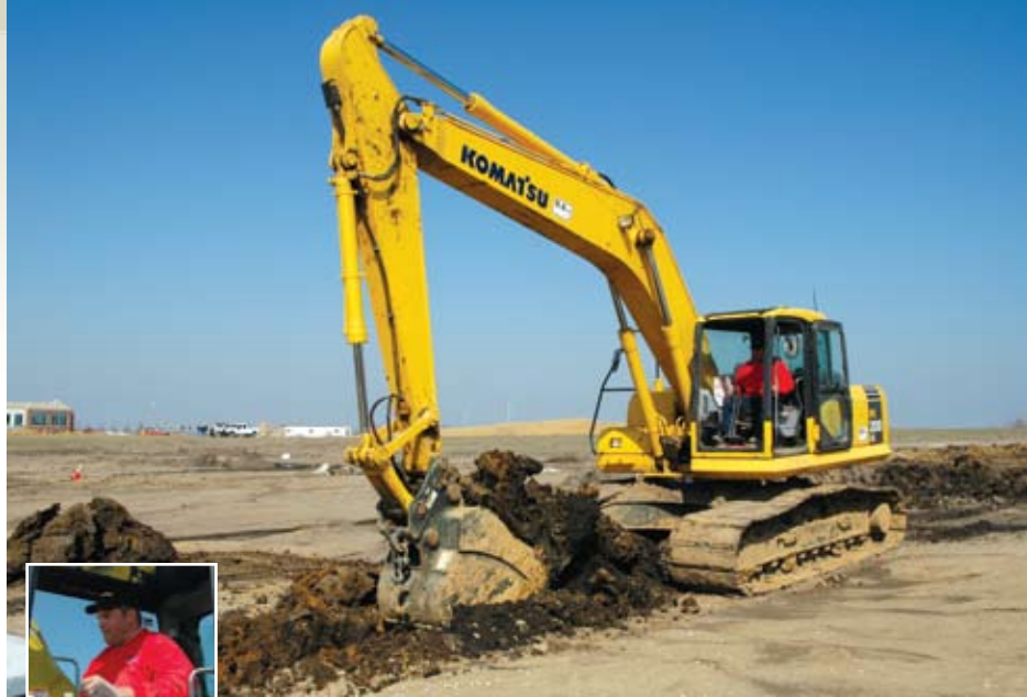
Mark McIntyre uses Heartland Midwest’s PC200LC-7 to dig a water line at The Bellagio, a commercial development in Leawood, Kan.
